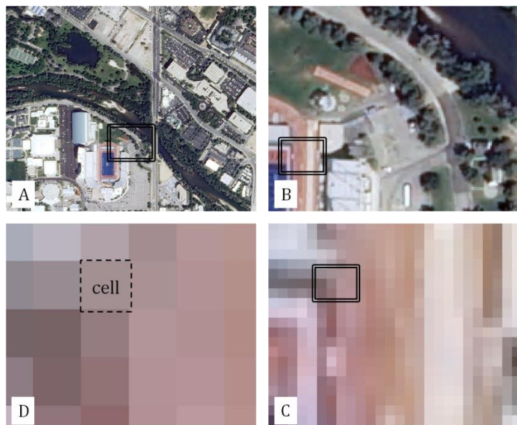
Figure 1.5. This raster displays an aerial image. The area in the black box in figure A is enlarged in figure B. The black box in figure B is enlarged in figure C. The black box in figure C is enlarged in figure D. One cell is labeled in figure D.
